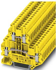
Double-level terminal block with screw connection, cross section: 0.14 mm<sup>2</sup> - 6 mm<sup>2</sup>, AWG: 26- 10, width: 6.2 mm, color: Yellow
